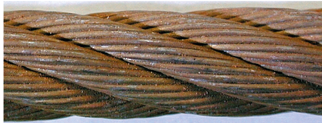
1. Beginning of surface oxidation, can be wiped clean, superficial – Rating: 0% towards discard
