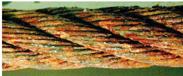
3. Surface of wire now greatly affected by oxidation – Rating: 60% towards discard
