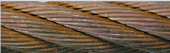
1. Beginning oxidation of the surface, can be washed off, only on the surface. Classification: 0 % of the discard maturity.
