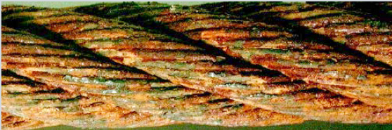
3. Surface heavily oxidized. Classification: 60 % of the discard maturity.
