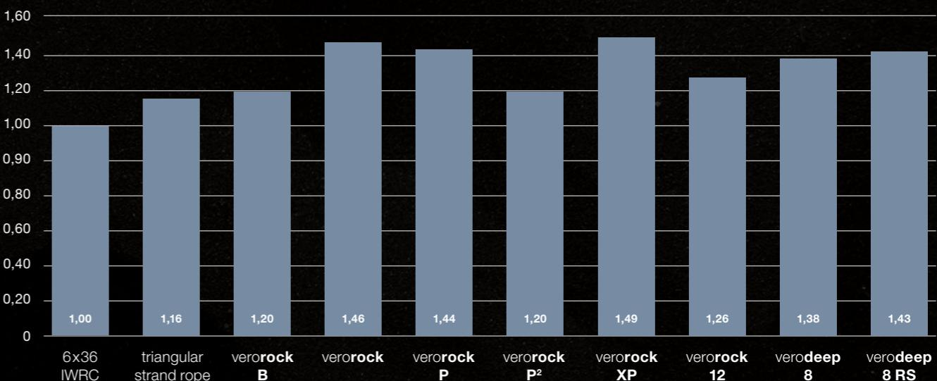
verope special mining ropes are designed to achieve high breaking loads and better strength-to-weight ratios. High ductility wires drawn to controlled tolerances are stranded and closed into a rope, constructed with optimized gap spacing between the individual rope elements.
