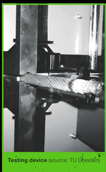
Additionally to tensile and bending loads, wire ropes are exposed to enormous traverse loads in multi-layer spooling. In order to be able to withstand these loads and to avoid spooling problems, a high degree of radial stability is needed. The radial stability of the rope also influences the deforming behavior of the drum.
