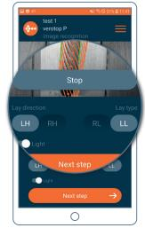
Place the rope on a lighter background within the provided frame until the green lines have detected the outer lines of the rope.
