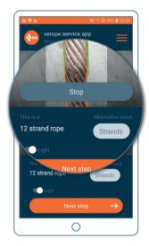
Place the rope on a lighter background within the provided frame until the green lines have detected the outer lines of the rope.
