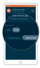
Please provide the rope strength and wire surface in addition and select the appropriate rope configuration from the list.
