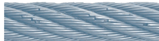
Figure 39: Condition at 60% of the bending cycle until breaking point
