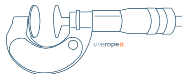
Figure 11: Micrometer with wide measuring flanks
