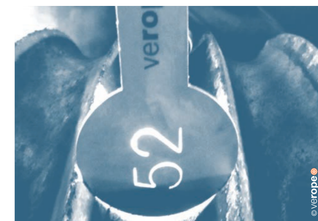
Figure 74: Groove gauge (shown in a too narrow groove)
