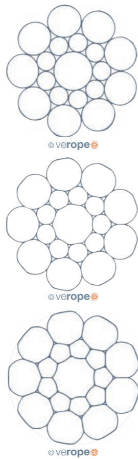
Figure 8: Uncompacted and compacted round strands
