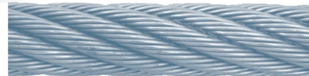
Figure 37: Condition at 20% of the bending cycle until breaking point
