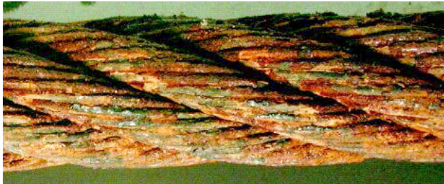
3. Surface of wire now greatly affected by oxidation – Rating: 60% towards discard
