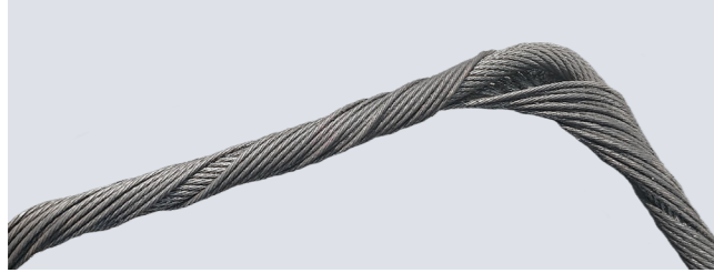
Protruded IWRC of rotation resistant rope
