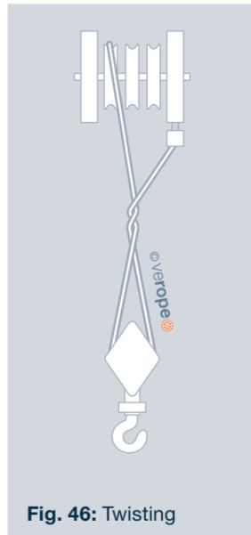
1. The reeving of an odd number of wire rope strands is significantly less stable than the reeving of an even number of wire rope strands. A 3-strand reeving is less stable than a 4-strand reeving.
