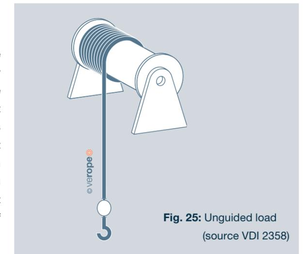
Fig. 25: Unguided load (source VDI 2358)
