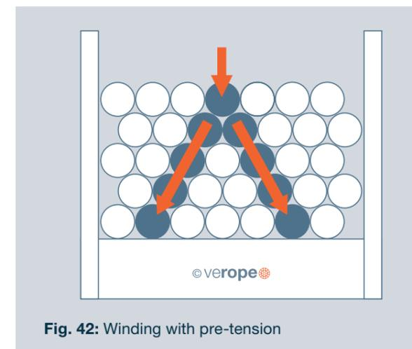
Fig. 42: Winding with pre-tension
