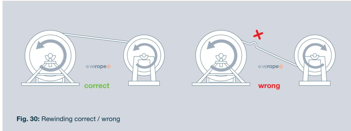
Fig. 30: Rewinding correct / wrong
