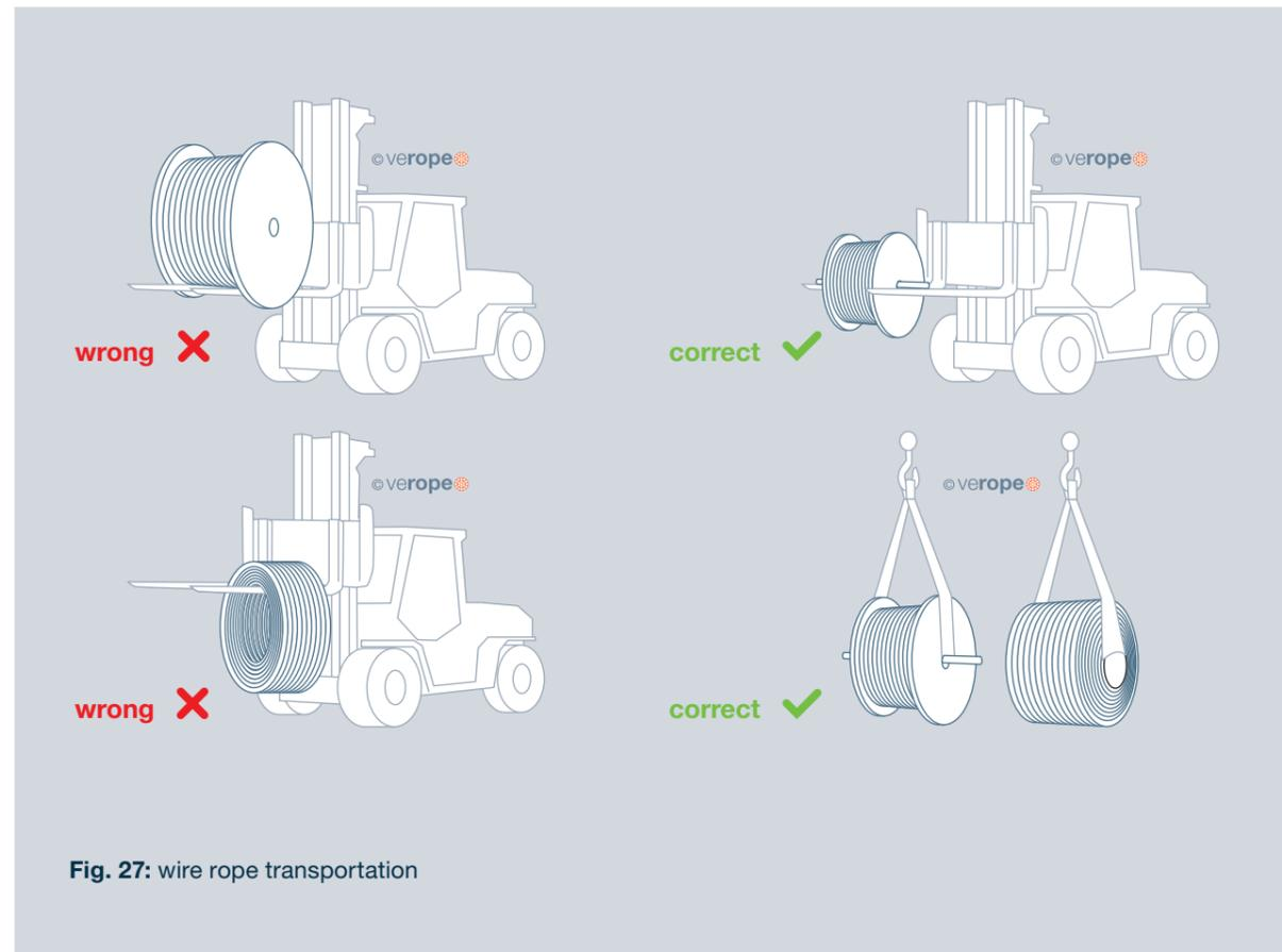
Fig. 27: wire rope transportation
