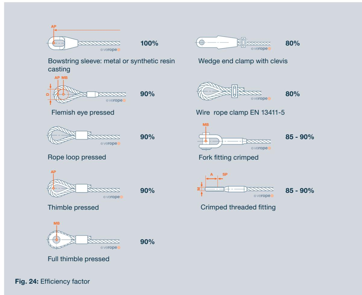
Fig. 24: Efficiency factor
