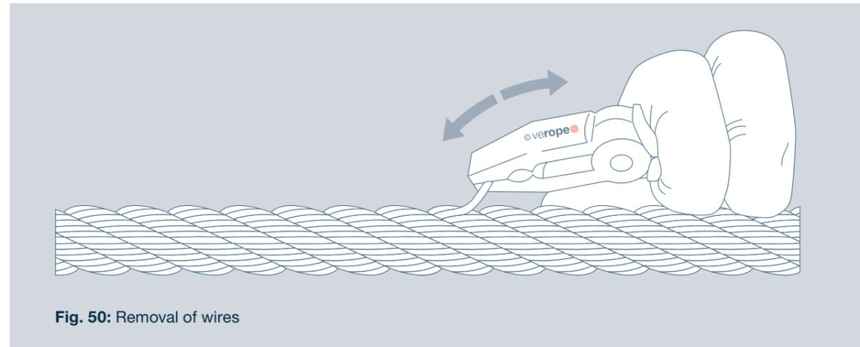
Fig. 50: Removal of wires
