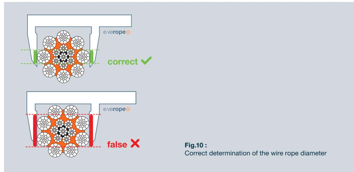
**Fig.10 :** Correct determination of the wire rope diameter
