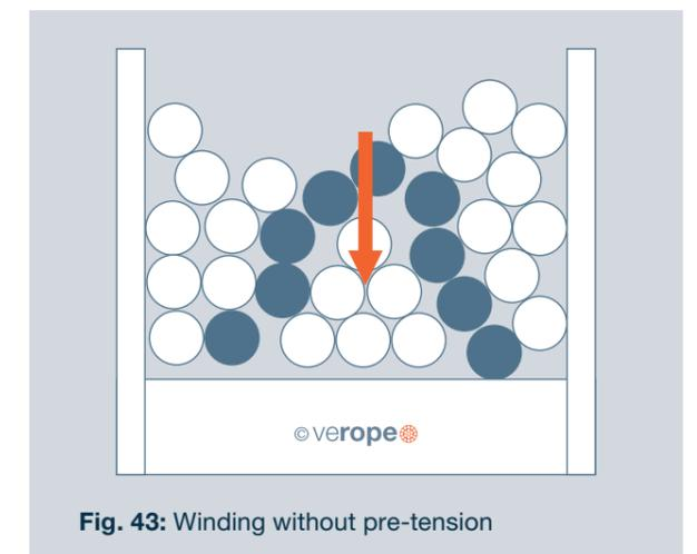
Fig. 43: Winding without pre-tension
