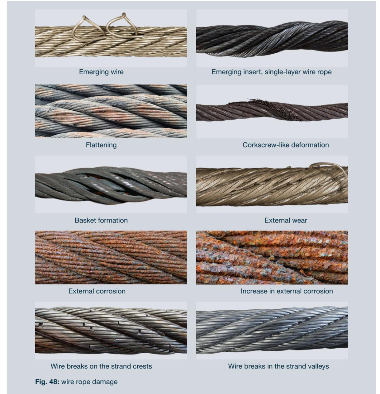
Fig. 48: wire rope damage
