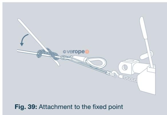
Fig. 39: Attachment to the fixed point
