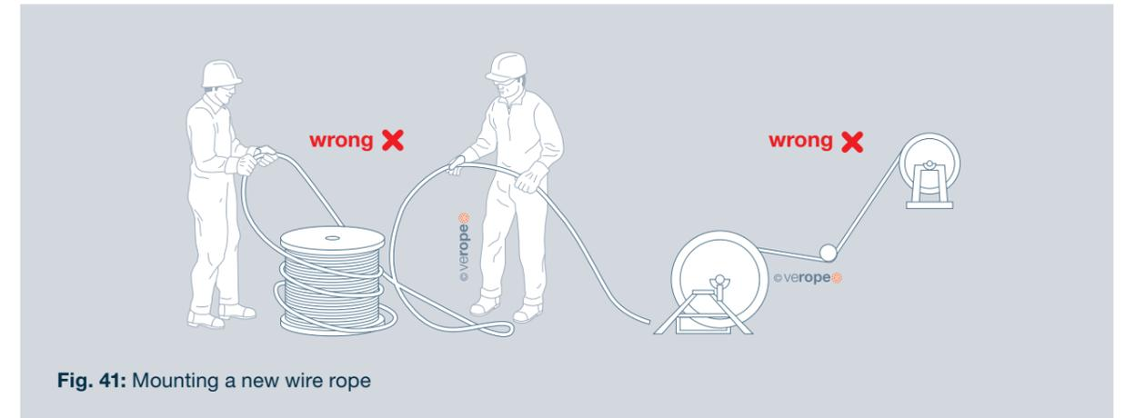
Fig. 41: Mounting a new wire rope
