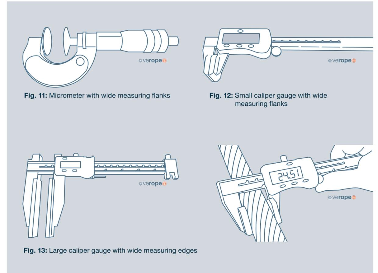
**Fig. 11:** Micrometer with wide measuring flanks
