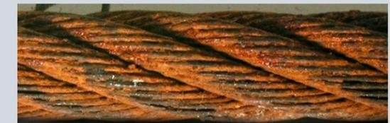
4. Surface badly pitted, wires without tension, gaps between wires. Immediate storage.
