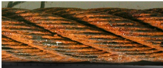
4. Surface heavily pitted and wires quite slack, gaps between wires – Discard immediately
