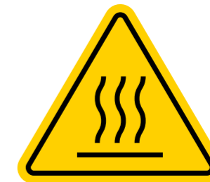
Danger / Caution / Burns
