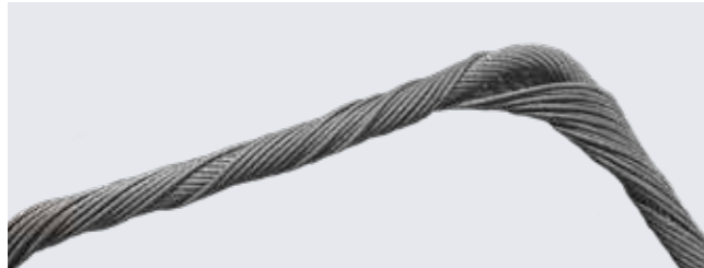
Protruded IWRC of rotation resistant rope
