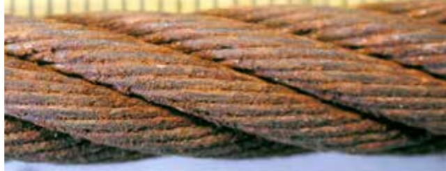
2. Wires rough to touch, general surface oxidation – Rating: 20% towards discard
