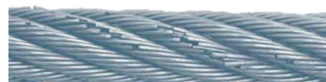
Figure 40: Condition at 80% of the bending cycle until breaking point
