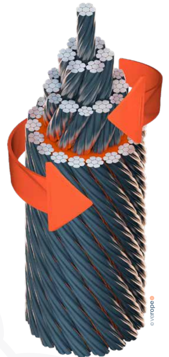
Figure 21: Rotation-resistant rope verotop P: the torques of the rope core and the layer of outer strands, generated under load, work in opposite directions.
