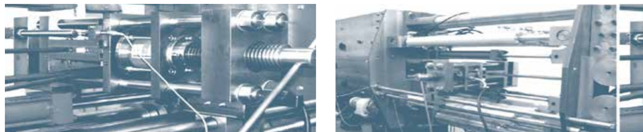
Figure 62: Testing principle of the measurement of the modulus of elasticity under load (source: TU Clausthal)
