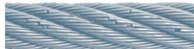
Figure 39: Condition at 60% of the bending cycle until breaking point
