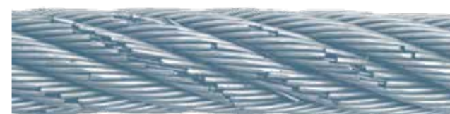
Figure 41: Condition at 100% of the bending cycle until breaking point
